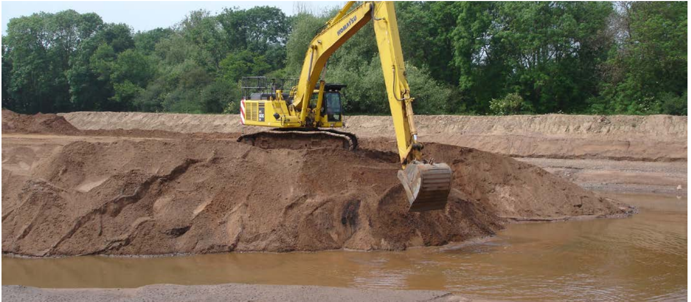
Working terrace sand and gravel deposits at Ball Mill Quarry (courtesy of Herefordshire and Worcestershire Earth Heritage Trust)
